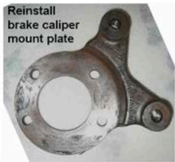
reassemble hub and brake rotor. Tighten bolts to 30#
