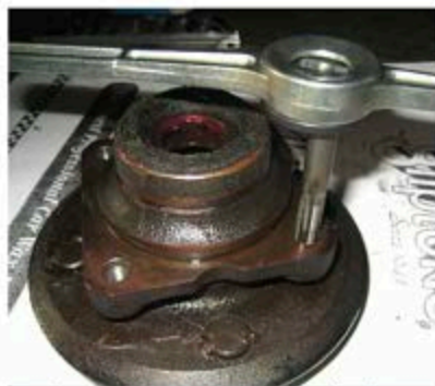
inner bearings installed
