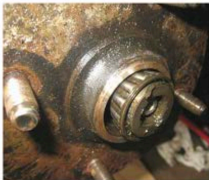
Outer Wheel Bearings Exposed
