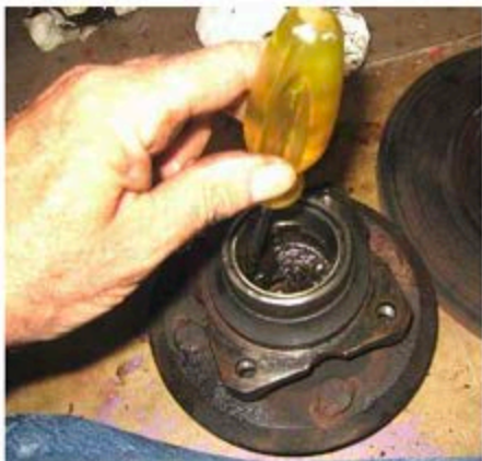
Photo above shows removing outer race.
