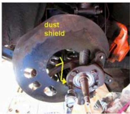
Remove 3rd dust shield bolt from caliper mount.
