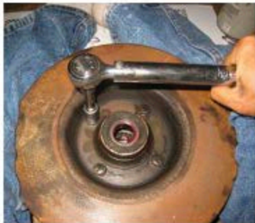
reassemble hub and brake rotor. Tighten bolts to 30#
