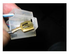
After removing the clip you will notice that the tab is flattened. Use the screwdriver or similar tool to bend it back out. If it is not sticking out it will not secure the clip in the plastic.
