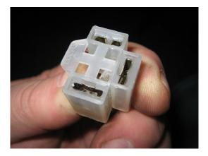
Insert a small screwdriver or similar tool in the notch along side the brass clip.
