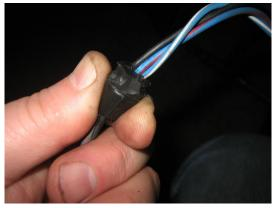
Then unplug the wires from the main harness in front of the radiator. This and other steps might be much easier if the shroud is removed.
