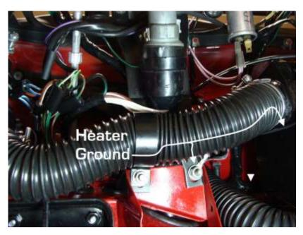
Early car heater motors have two white wires with one of them exiting the heater case as the ground wire along with the low and high speed wires.
