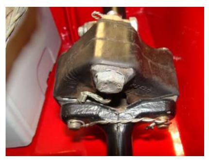
The jumper strap bonds the lower steering column to the upper column.
