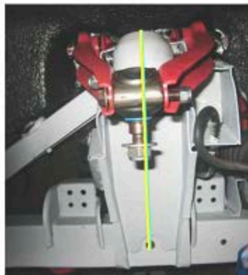
Dry fit ball joint to confirm offset to rear of car
