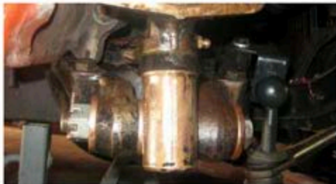
Trunnion Degreased to show Details
