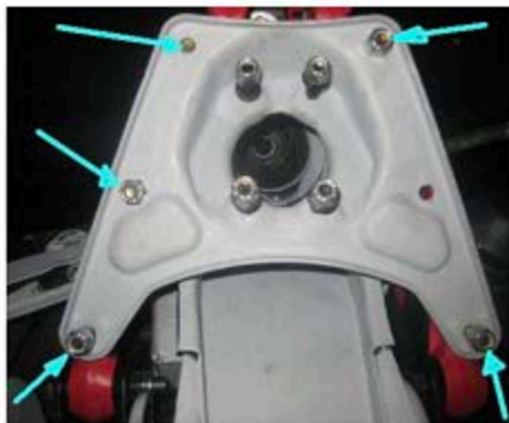
COIL SPRING PAN DRY FIT INSTALLED - As viewed looking up from floor level.
