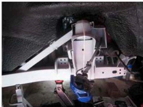
Frame refurbished - ready for new suspension
