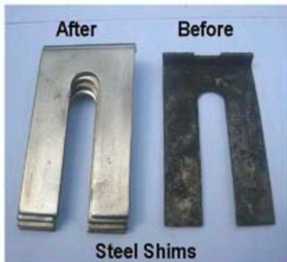
ALIGNMENT SHIMS - REFURBISHED
