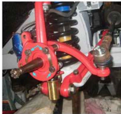
DRY FIT READY TO TORQUE BOLTS. STEERING ARM AND TIE ROD END SHOWN
