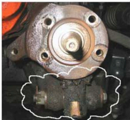
Trunnion prior to removal
