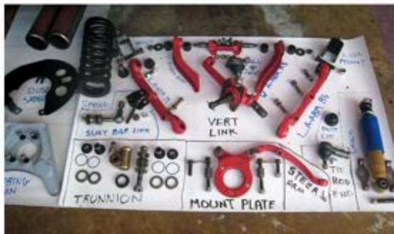
NEW FRONT SUSPENSION READY TO INSTALL:
