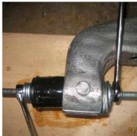
STARTING INSTALL NEW T/A BUSHING
