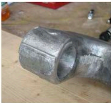
Ready to Install First New Rubber Bushing
