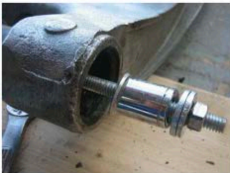
Bushing tool with socket extension to complete Removal of old rubber bushing.
