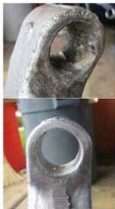
Bushing Hole- before / After Deep Cleaning
